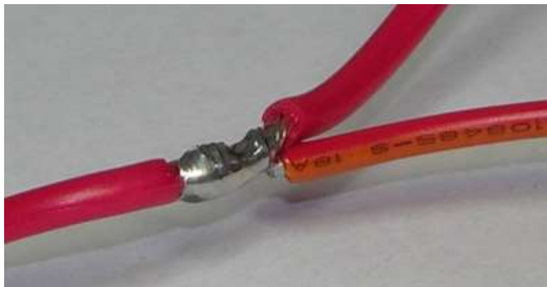
Figure 4: Correctly Soldered Connection
