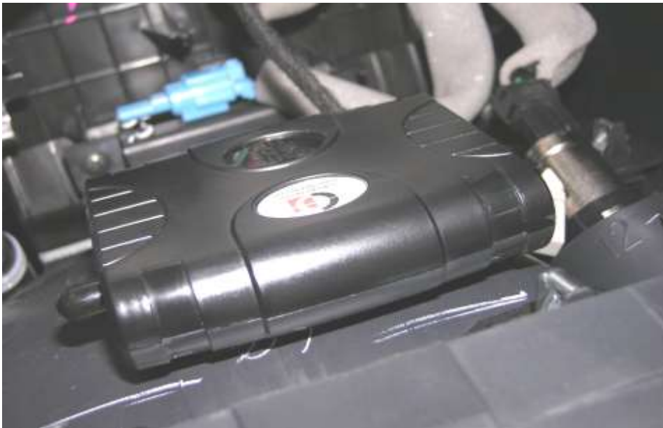
Figure 12: Ensuring the Device is Located with 30cm Free Radius
