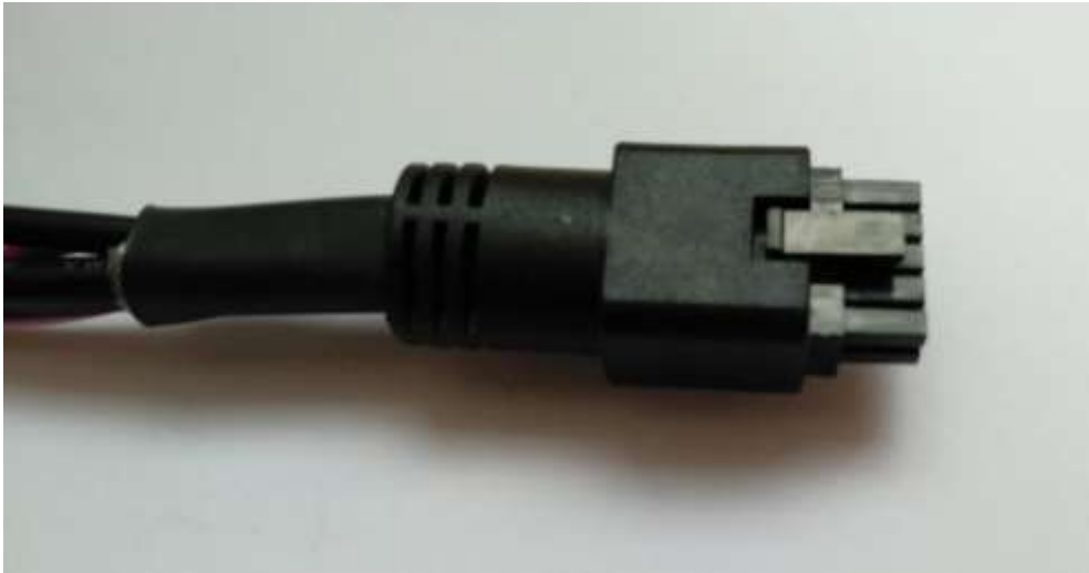
Figure 14: Harness 10 Pin Connector and Latch
