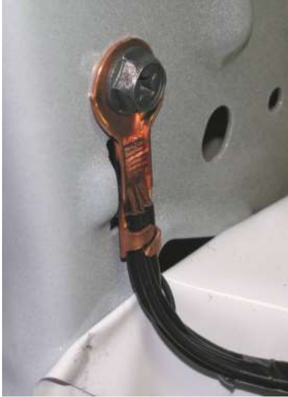
Figure 9: Connecting Negative Power Wire
