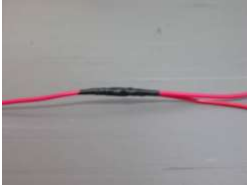
Figure 5: Isolate the Connection
